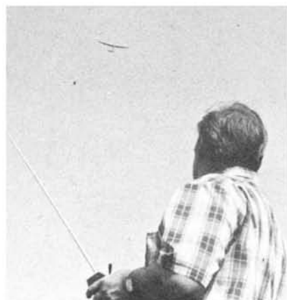
Russ Glasgow brings the K8B overhead for the camera. This ship is a floater with light wing loading. Add weight for slope soaring.
